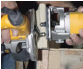
Figure 1. For the look of a traditional stool, the author uses full 1-inch-thick stock profiled with a router. He shapes the bottom edge with a cove-and-bead bit and the top edge with a 5/16-inch roundover bit. At right, the finished edge profile with the router and trimmer held in place.
